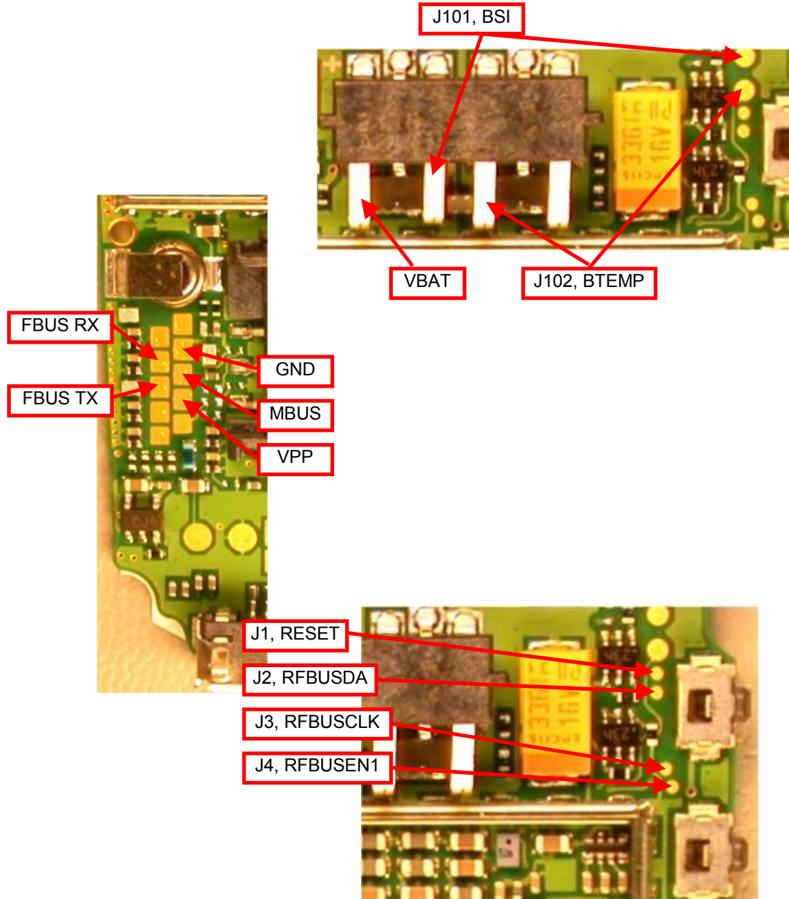
Figure 50: Flash programming testpoints
